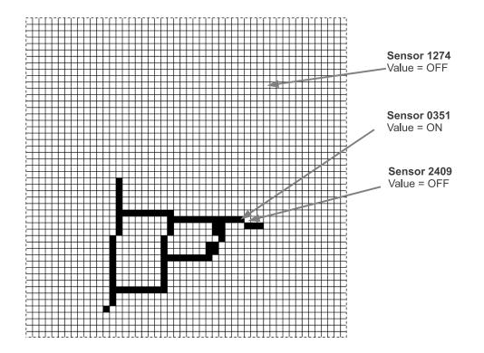
FIG. 2.2. A sensor grid. We've arranged the 2,500 sensors in a 50 by 50 grid, though the computer doesn't have this ordering knowledge. In this example, 78 of the sensors are ON (including Sensor0351), and the other 2422 sensors are all OFF. We also allow that a sensor can be "UNSPECIFIED".
