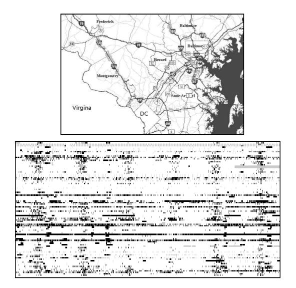
FIG. 1.1. Traffic speed sensor data. The top image is a map of automobile traffic speed sensor locations. Below, is a time series of the traffic values taken every 5 minutes for a week. The y axis are the 87 sensors in an arbitrary order. The x axis is time. Black areas are where the average traffic speed over the 5 minute window is less than 25 miles per hour. Grey areas are missing data. We can see the morning and evening rush hours as dark evenly spaced bands.
