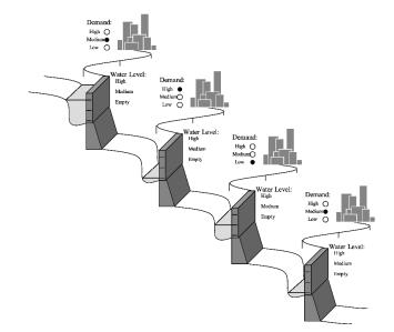
FIG. 3.11. A sequence of hydroelectric reservoirs and dams. Each of the 4 dams provides power for a single city. Each city's demand (and pay rate) varies with time. The agent must choose which dams to keep closed or open to produce electricity to sell immediately to its city. Opening a dam also sends some water to the next reservoir downstream. There is assumed to be a steady flow of water into the first reservoir.
